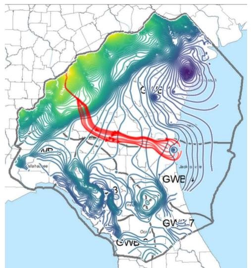
Figure C-3. Simulated heads from NFSEG Layer 5 (blues and greens, modified from Durden et al. 2019) and pathlines (red) for flow to the pumping center near Jacksonville.
